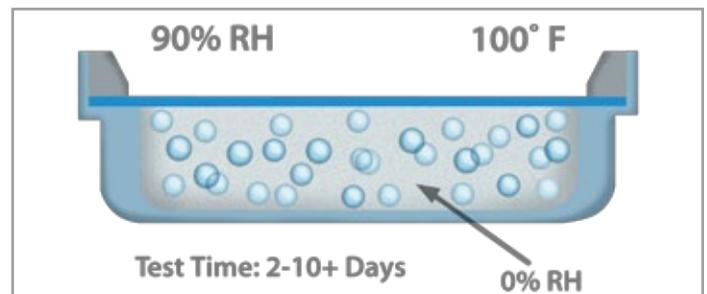
During the gravimetric test, a cup or dish is filled with desiccant or water, placed in a temperature and humidity controlled chamber, and weighed periodically. Depending on the barrier properties and sample thickness, the gravimetric method could require a test time of one day to two to three weeks (or longer). Enough data points should be collected until weight gain (or
